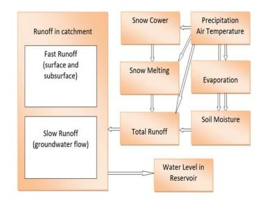
Fig. 6. Schematic picture of the hydrological model ILHM.
